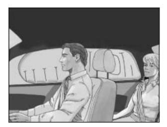
If your vehicle has a side impact airbag for the right front passenger and the person seated directly behind that passenger, it is in the ceiling above the side windows.
